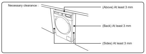
For neater installation under the counter, check the height of internal measurement before fitting and adjust to the appropriate height with the adjustable feet.
