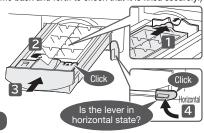
When the frame for the ice tray cannot be pushed into the back, the motor that drives the ice-tray may have operated. Remove the ice tray once and then push the frame alone into the back, and then touch leaves button with all the doors closed to turn on "Off". After 1 minute, the ice-tray driving motor gets ready, allowing you to mount the ice-tray.
