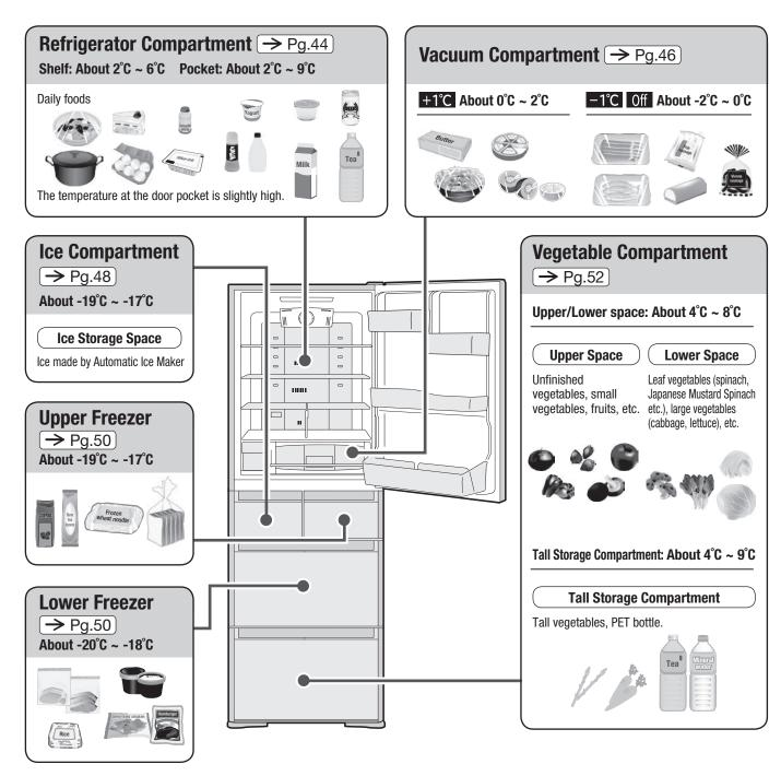
The above temperatures are standard values under the condition that the refrigerator is stable with no food stored and the doors closed, at ambient temperatures of approximately 32°C, whereas the setting is "for both refrigerating chamber and freezing chamber.
