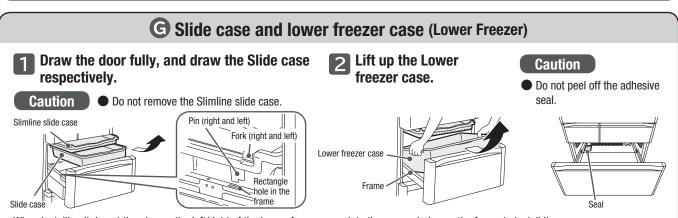
When installing it, insert the pins on the left/right of the Lower freezer case into the square holes on the frame to install it. Moreover, hitch the fork on the left/right of the Slide case to the outside of the Lower freezer case.
