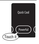
Touch MENU button to turn on the indicator lamp, and then touch Powerful button to turn off "Quick Cool" indicator lamp.
