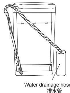
Unplug U-shaped hose and insert into water drainage hose.
