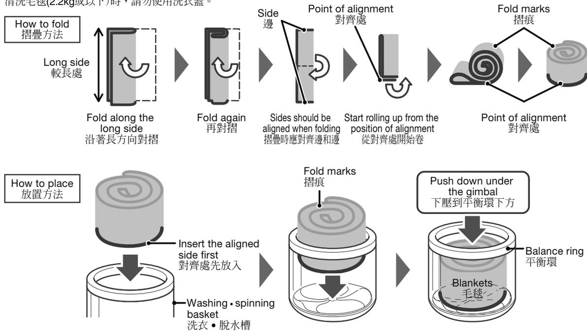
If the aligned side of blankets are not inserted into the washing • spinning basket first, blankets may be damaged during operation.
