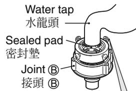
Tighten screw in advance if it is located close to the wall. 靠近牆壁的螺釘，可預先用手擰進一些。
