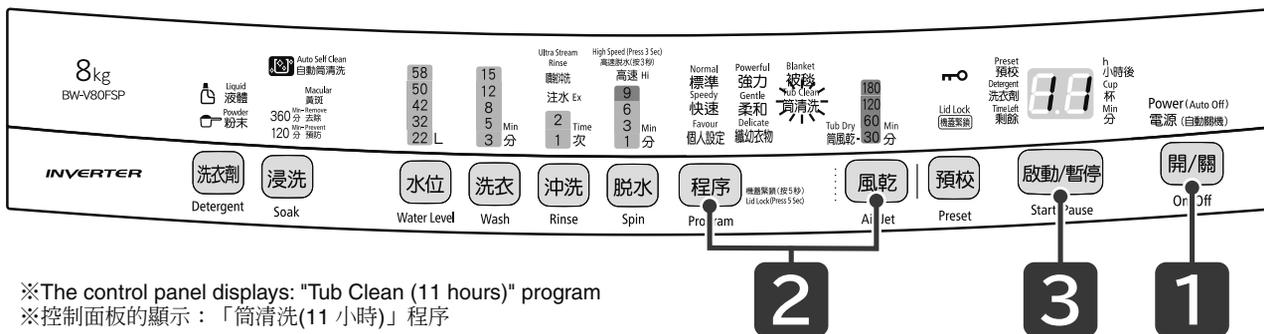
※The control panel displays: "Tub Clean (11 hours)" program
