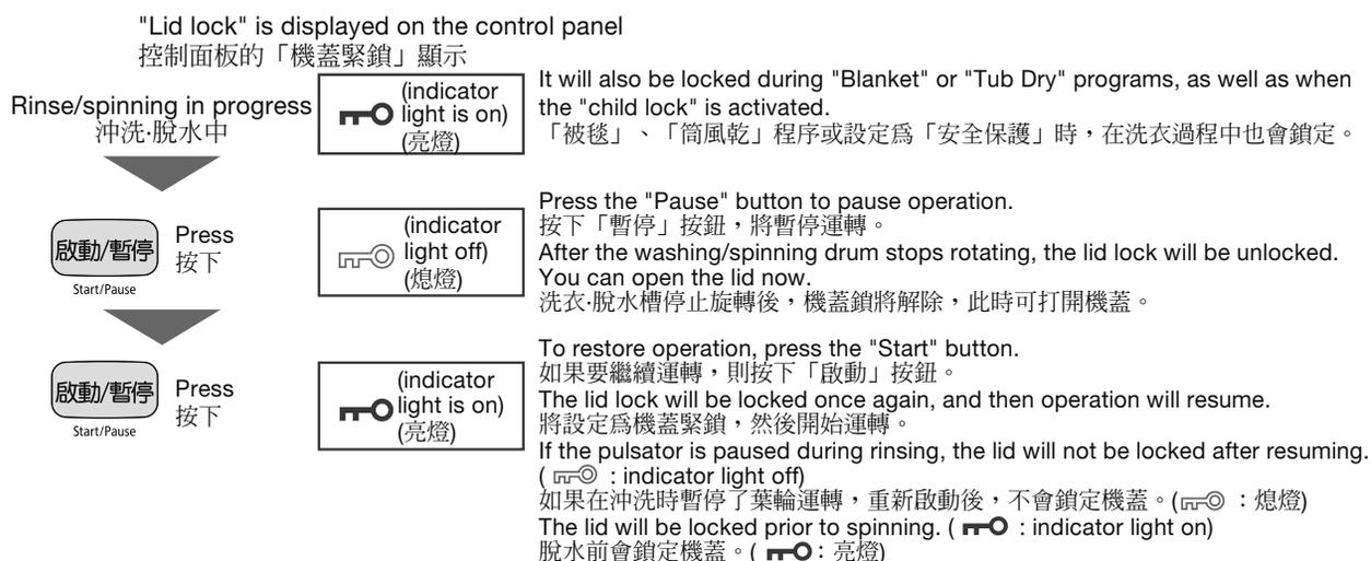
If power is cut off during operation, the lid will remain locked and operation will cease.
