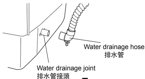
**2** After the connection is completed, please use hose clipper to clamp the water drainage hose to avoid fall-off.
