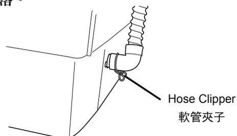
**3** ① Insert the fixing holder of water drainage hose into claws clasp on either side of back side of top cover.
