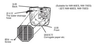
Align the hook on the base plate with the square hole on the chassis and insert it, then tighten the screw.
