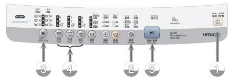
■ Any of the programs of "Washing", "Rinsing" and "Spinning" can be set up alone, and the programs can also operate in combination. (The content of the washing will not be stored) 可以單獨設定洗衣、沖洗、脫水任何一個程序,亦可將各個程序組合運轉。(洗衣內容將不會被儲存)
