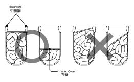
Put the laundry into the spin dryer basket evenly, and set the Inner Cover horizontally inside the basket by putting it under the bottom of the balancer.
