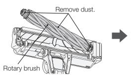
Remove tangled lint and similar types of dirt in the groove using tweezers, etc.
