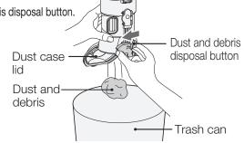
Remove attached dust and debris.
