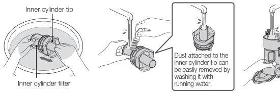
Move the inner cylinder tip in the direction of the arrow and wash with water.
