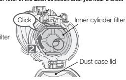
Note If the filter is not securely attached, it might fall when you empty the dust case. Similarly, if you use the vacuum cleaner without securely attaching the filter, strange sounds might come from around the filter.
