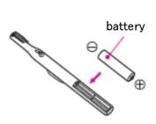
Fit the cutout part of battery cover to the switch part, and make sure the battery cover closed firmly.
